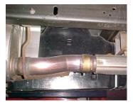
LAY OUT THE GIBSON EXHAUST ON THE FLOOR SO IT LOOKS LIKE THE DRAWING. COMPARE PART NUMBERS WITH MANUAL. TO REMOVE YOUR STOCK EXHAUST, REMOVE IT FROM THE CLAMP LOCATED JUST IN FRONT OF THE MUFFLER. YOU MAY NEED TO HEAT IT UP FOR EASIER REMOVAL. NOW CUT OFF YOUR STOCK TAILPIPE JUST BEHIND THE MUFFLER. USE WD-40 TO AID IN THE REMOVAL OF HANGERS. LEAVE ALL RUBBER GROMMETS IN PLACE.
