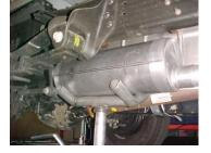
INSTALL MUFFLER #B ONTO HEADPIPE 1 ½" TO 2". MUFFLER OUTLETS SHOULD BE ON TOP. ROTATE UNTIL LEVEL. SUPPORT MUFFLER WITH A JACK STAND. NEXT, INSTALL FRONT MUFFLER HANGER #F INTO RUBBER GROMMETS, LOCATED NEXT TO MUFFLER INLET. THIS CLAMP WILL ALSO BE USED TO SECURE MUFFLER TO HEADPIPE. DO NOT TIGHTEN.
