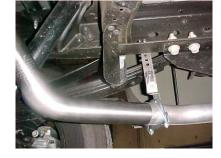
INSTALL PASSENGER SIDE OVERAXLE PIPE #C INTO MUFLER 1 ½" TO 2". USE CLAMP # I TO SECURE. DO NOT TIGHTEN. ROTATE UNTIL PIPE TOUCHES HANGER. USE CLAMP #I TO HOLD PIPE TO HANGER. DO NOT TIGHTEN.
